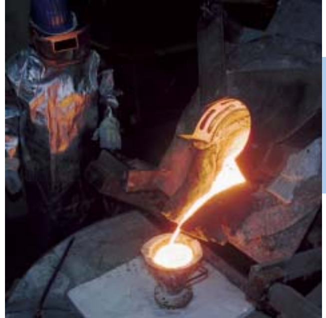
Filling the liquid metal into the atomizing funnel.
