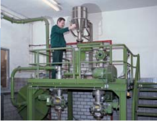
Wind screening for the powder grain size.
